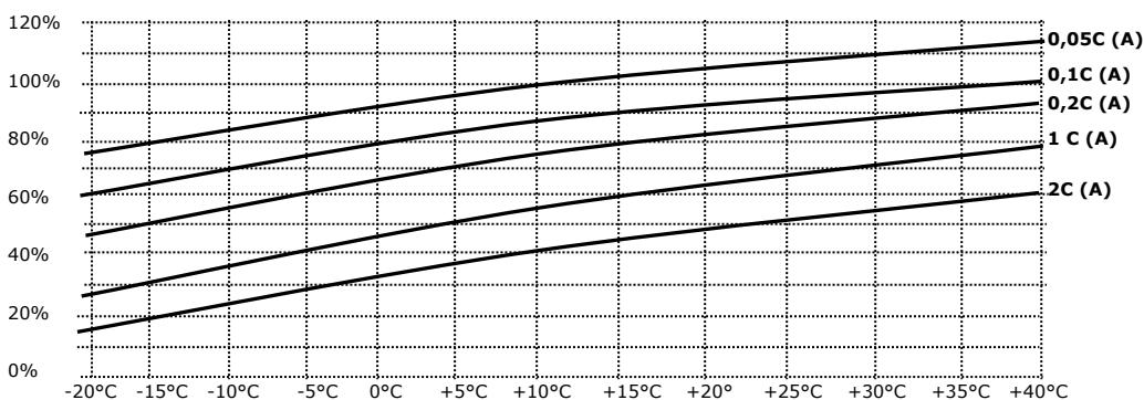
A low temperature reduces remaining capacity.
