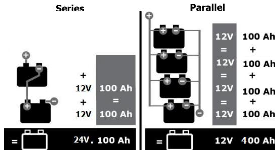
NB: Cables resistors in every chain need to be the same (same section, same length).
