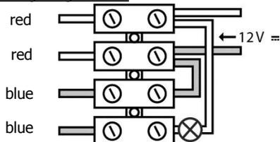
Nb: the voltage of the light must be identical to that of the motion detector.
