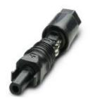
Photovoltaic connector, Range of articles: Sunclix, Connector, color: black, number of positions: 1, min. conductor cross section: 2.5 mm², max. conductor cross section: 6 mm², rated voltage: 1100 V DC, rated current: 35 A, Connection method: Spring-cage, Type of contact: Socket, min. cable diameter: 5.5 mm, max. cable diameter: 8 mm
